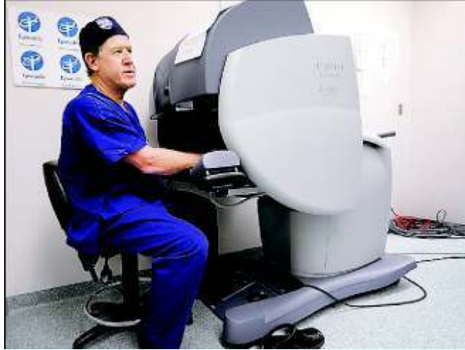
▲ Remote control: Tony Costello performs a prostatectomy by machine, guiding the robot's arms from his console a few metres from the operating table.
